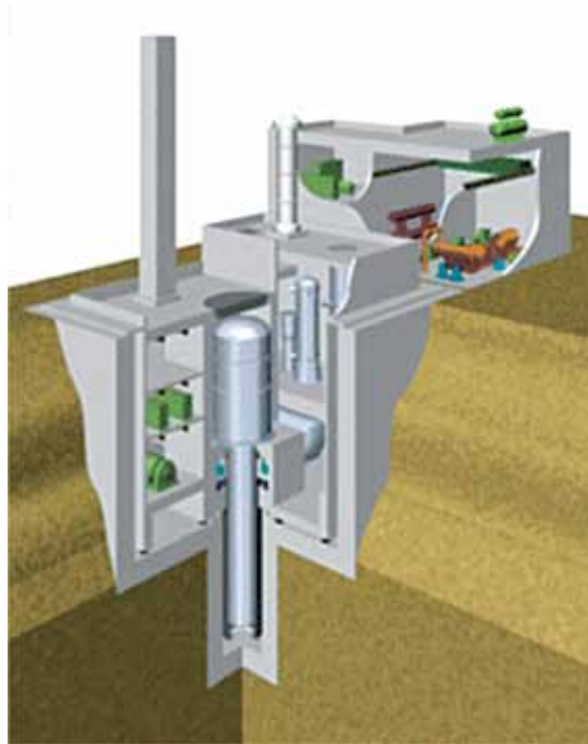
Toshiba 4S sodium-cooled small reactor, is intended to be operated underground with a turbine building on the surface, and has an electrical output of 10 MWe (30 MWt).
