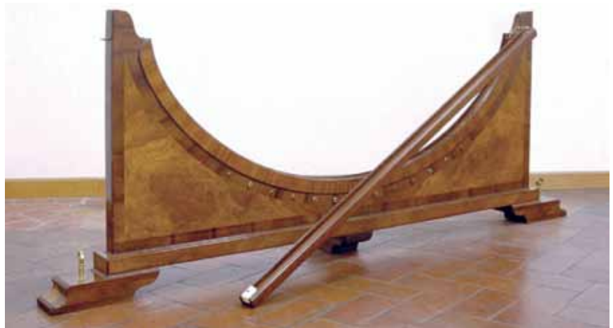
A ball rolling down the pictured cycloid curve will always arrive at the bottom before a ball rolling down a straight path.
