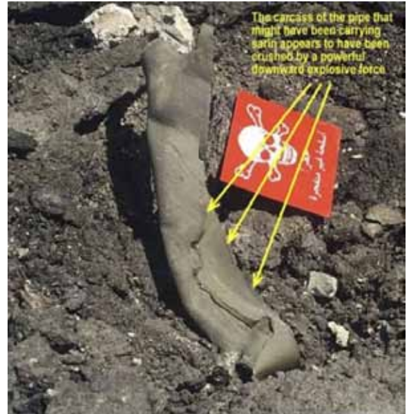
Deformation of sarin containing pipe and crater from the action of the explosive charge placed on top of the pipe.
