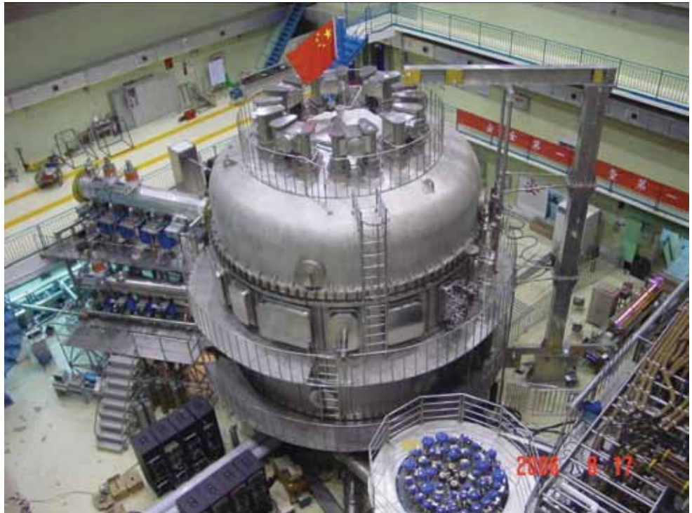
China’s work on the frontiers of science includes thermonuclear fusion power. Here, China’s EAST fusion reactor, the first fully superconducting Tokamak in the world.
