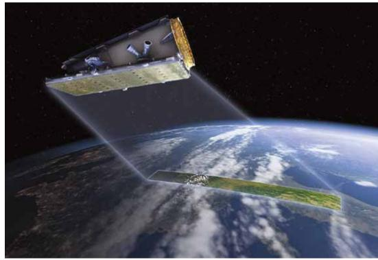
Space technology is not just for industrialized economies, Dr. Mohammed insists. Shown: a Synthetic Aperture Radar (SAR) Satellite System, NovaSAR-s, manufacted by Surrey Satellite Technology Ltd, used by Nigeria.
