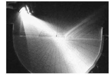
In an experiment conducted by the LYM, the path of light is seen to change direction when it passes from air to water.
