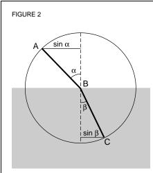
Snell determined that the ratio  $\sin/\alpha : \sin/\beta$ is maintained for two media, no matter at what angle the light hits the boundary.
