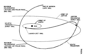
The Ulysses spacecraft is now on its way to a February 1992 encounter with Jupiter. A Jovian gravity assist will boost it south of the planetary plane of the ecliptic to place it under the Sun's south pole in mid-1994. One year later, it will view the Sun from above its north polar region.
