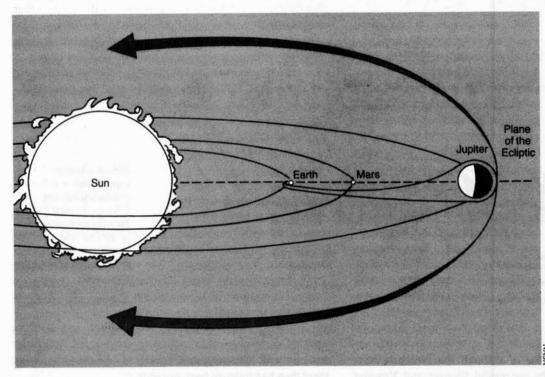
The two-spacecraft International Solar Polar Mission: According to the original plan, two spacecraft, launched simultaneously from the Shuttle, would have orbited the poles of the Sun at the same time. Thus, a genuine threedimensional view of the Sun would have been possible.
