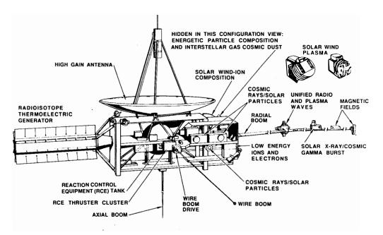
Eleven scientific experiments will be conducted aboard Ulysses, to shed light on the magnetic structures of the Sun, the production and propagation of the solar wind, and characteristics of the interplanetary medium.
