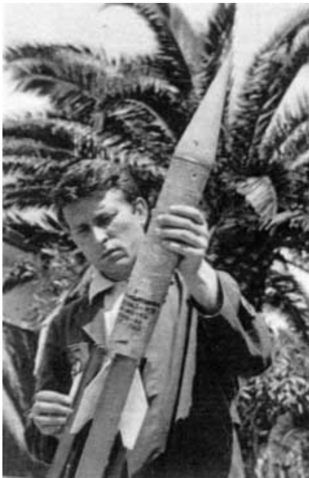
The indigenously-developed Slovenia Kamnik-1 rocket was used to seed clouds and suppress the formation of hail during thunderstorms. The program, itself, was later suppressed by the Yugoslav military.
