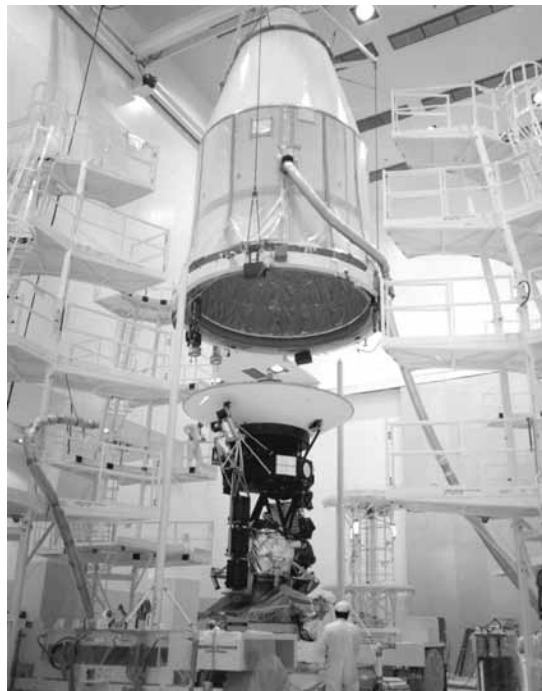
The protective launch shroud is lowered onto Voyager 2.
