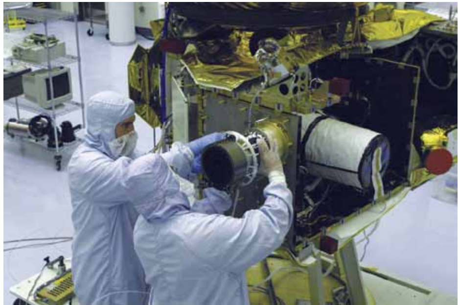
NASA/Johns Hopkins University Applied Physics Laboratory/Southwest Research Institute SWAP (Solar Wind Around Pluto instrument) being installed on the New Horizons spacecraft, on March 8, 2006. It will provide scientists with a picture of the character of the solar wind, three billion miles from the Sun, and its interaction with Pluto's atmosphere.
