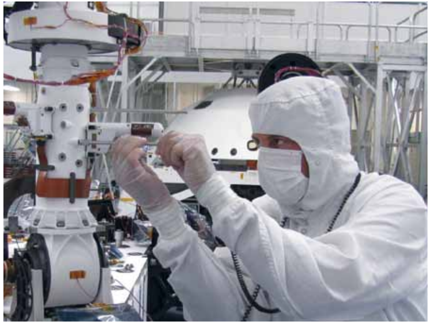
Man's mission on Mars requires a shift from merely human sense-perception, into the domain of universal physical principles as such. Here, weather sensors from Spain are installed on the Mars rover Curiosity, in September 2011, prior to its voyage to the Red Planet.
