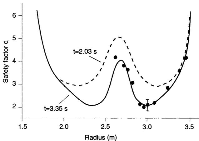
*Safety factor  $q$  profiles for TFTR at two different times, center of core is at approximately 2.65 radii on the major radius. The two low points of the W-shaped curve are where the shear reverses.*
