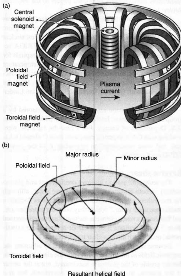
*This artist's rendition of a typical tokamak fusion device (a), shows the magnets and plasma current. The bottom schematic (b) shows the configuration of the magnetic fields within a tokamak, in which the magnetic fields confine and heat plasma inside of a donut-shaped vacuum chamber. Within the plasma, the toroidal and poloidal magnetic fields combine to produce helical fields.*
