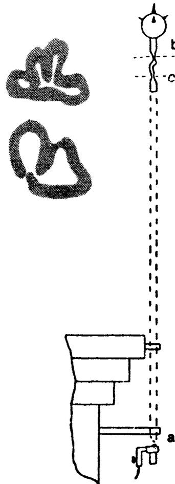
*Drawings of the cross-sections of the copper lightning rod that was crushed by the passage of a lightning bolt.*
