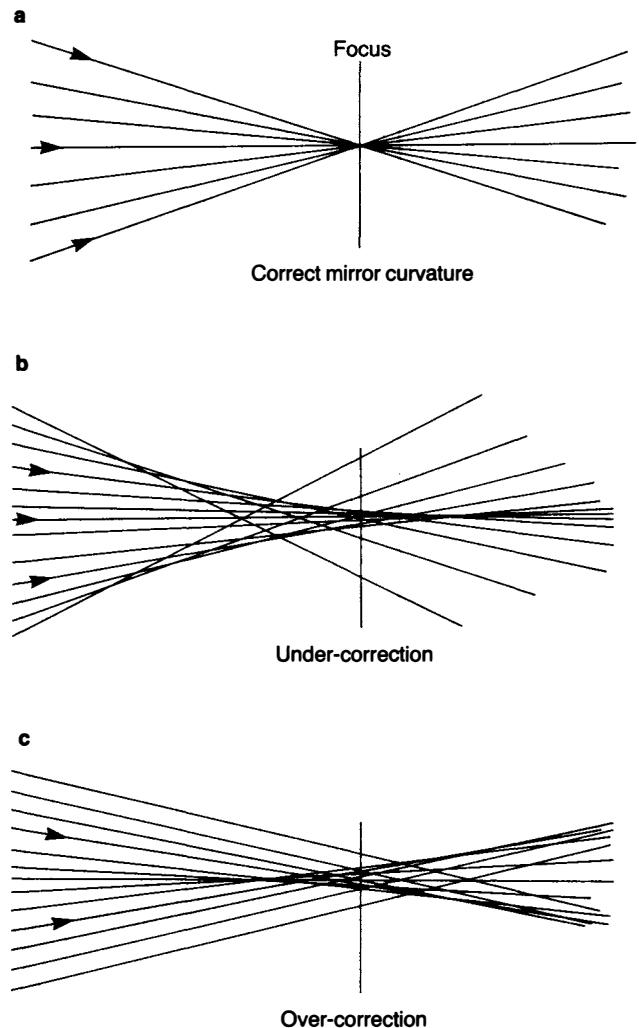
*A telescope's mirror or lens system must bring all points in the image into focus at a single focal plane (a). Mirrors or lenses with spherical aberration cause rays reflected from outer portions of the optic to come to focus (b) in front of, or (c) beyond, the focal point of the inner rays. Deviations toward the spherical produce the former result (so-called "under-correction"), but the term spherical aberration is applied to both cases.*
