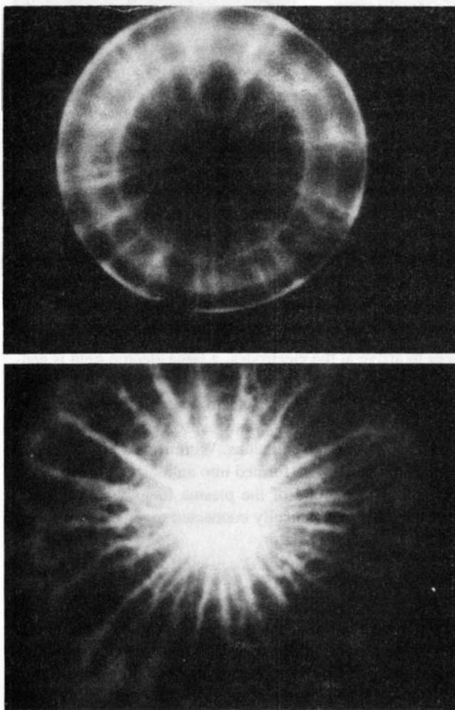
*The inner electrode is located at the circle at the center of the sheath. The outer electrode is located at the circumscribing circle. Barely visible in these photographs, as pairs of radial lines, are pairs of plasma vortex filaments which carry the electric current between the plasma focus electrodes.*
