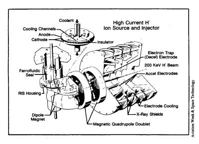
At the Los Alamos federal laboratory, the Defense Advanced Research Projects Agency (DARPA) is developing a rotating ion source and injector which produces continuous-wave beams of negative hydrogen ions. The beams are used in neutral-particlebeam research, essential to developing beam weapons for antiballistic-missile defense.
