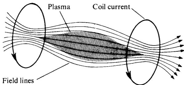
There are two main types of systems for magnetic confinement of plasma, one a closed system, as in the toroidal configuration employed in tokamak devices, the other an open-ended configuration like the simple "mirror" system above.
