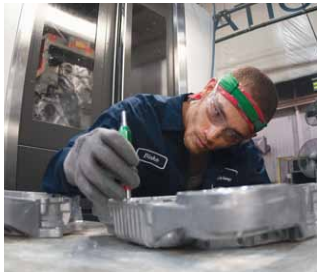
A Computer Numerical Control machine operator makes a process inspection after a casting is machined.
