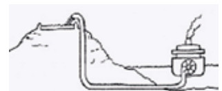
A concrete reservoir is placed at the top of the hills overlooking the coastline.
