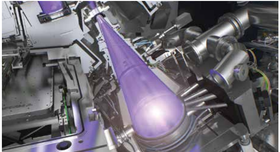
Inside ASML's TWINSCAN NXE3400C extreme ultraviolet (EUV) lithography machine, used for producing advanced (7 and 5 nm) microchips. Shown is the EUV source vessel. The U.S. blocked a Chinese company from buying one.
