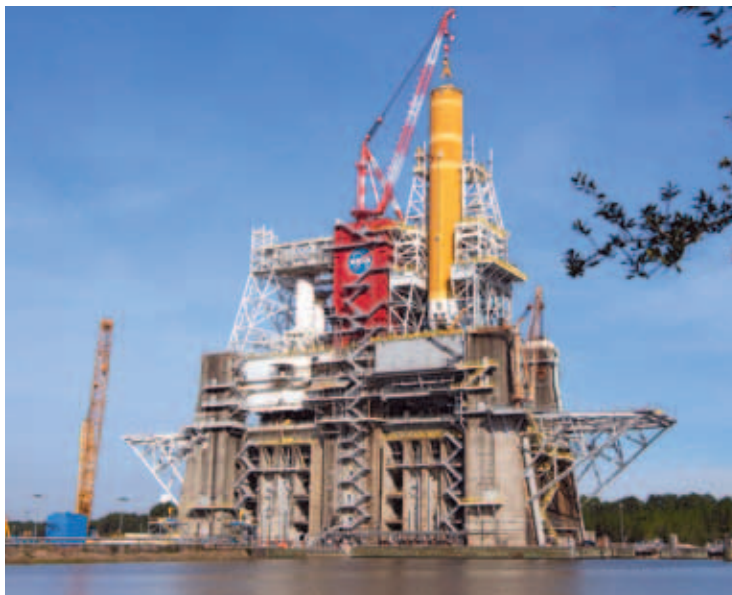
The core stage of the first Space Launch System (SLS) rocket being prepared for a test firing by the end of this year. It will launch an unmanned Orion spacecraft around the Moon next year on its first test flight.
