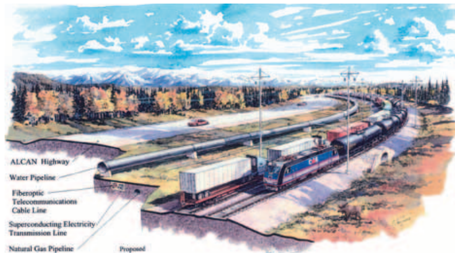
Artist's concept, showing a proposed rail, highway, utilities, and pipeline corridor near Lake Kluane, Yukon. Commissioned by Cooper Consulting for the Canadian Arctic Railway Company, which proposes to provide the missing links to connect Canada and Alaska to the proposed Bering Strait tunnel.
