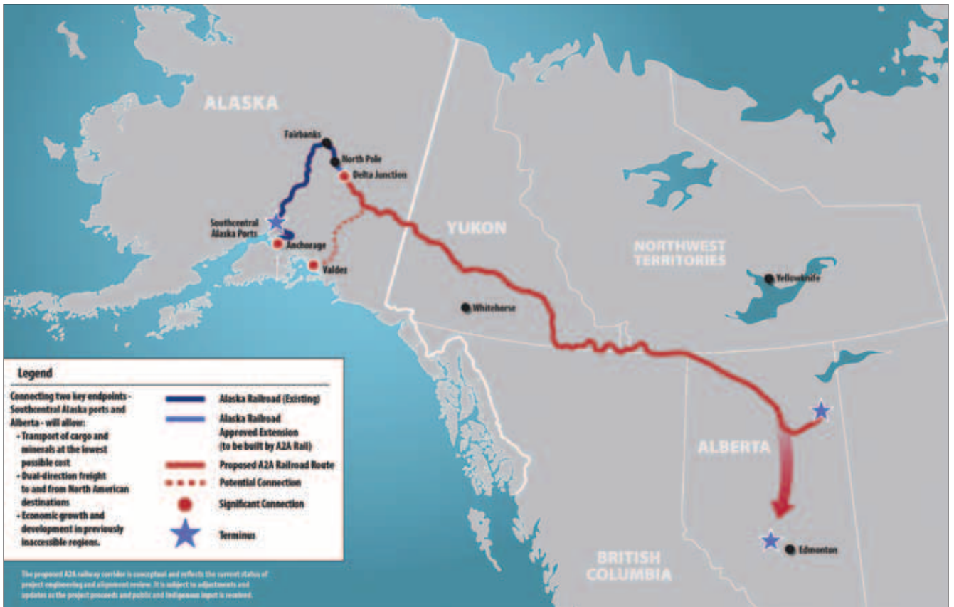
The proposed 2,570 km route of the A2A will connect at Delta Junction, Alaska to an upgraded Alaska Railroad mainline leading south to Alaska's deep-water ports; and at Fort McMurray, Alberta, to existing Canadian railways that serve the lower 48 states.
