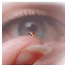
Lawrence Livermore National Laboratory An inertial confinement fusion fuel microcapsule. It is two millimeters in diameter and contains a central reservoir of deuterium-tritium (D-T) gas mixture, a frozen D-T solid-fuel layer; and an outer ablator layer.
