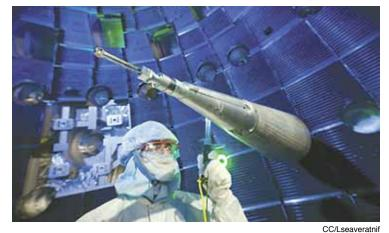
A technician works on a target positioner inside the National Ignition Facility (NIF) target chamber.
