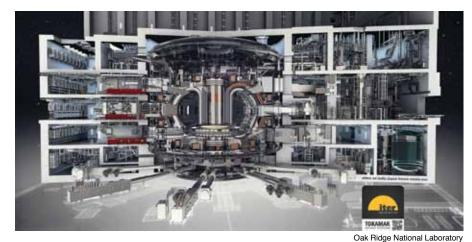
A cut-away drawing of the ITER tokamak and plant systems.
