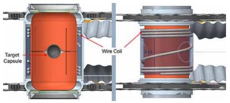
Lawrence Livermore National Laboratory Conceptual diagrams of a NIF hohlraum fitted with a B-field (magnetic-field) coil.
