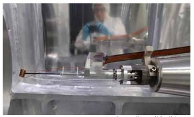
Lawrence Livermore National Laboratory A coil-wrapped hohlraum target installed at the end of a NIF diagnostic instrument manipulator.
