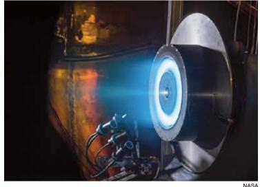
Prototype Hall thruster in testing at NASA's Glenn Research Center in Cleveland, OH. Four of these thrusters will used for maneuvering the Gateway in Lunar orbit.
