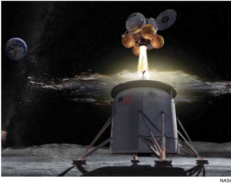
Artist's rendering of an ascent vehicle separating from a descent vehicle and departing the lunar surface.
