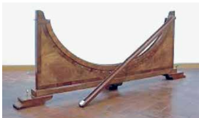
(a) A brachistochrone model built by Francesco Spighi in the 17th Century. A ball that rolls down the cycloidal track reaches the bottom faster than one rolling down the straight track.
