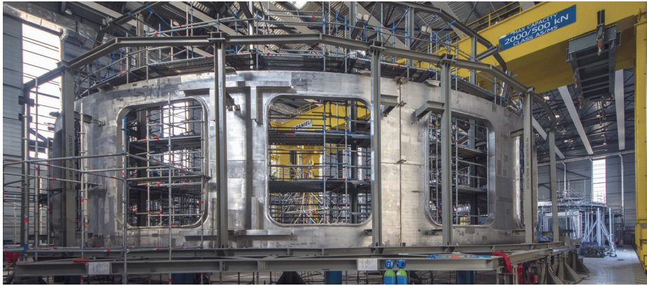
A higher level of cooperation in solving the issues that determine the future of mankind is needed. A cooling cylinder of the ITER fusion device now under construction in France.
