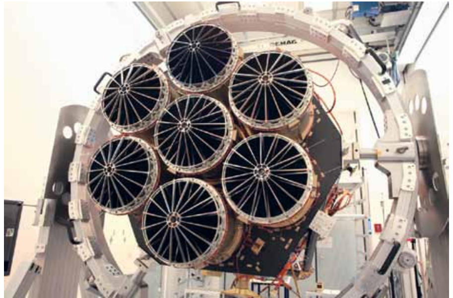
The eROSITA telescope, consisting of 7 identical mirror modules, will conduct the first complete sky survey in the medium X-ray range. It was launched July 13, 2019.
