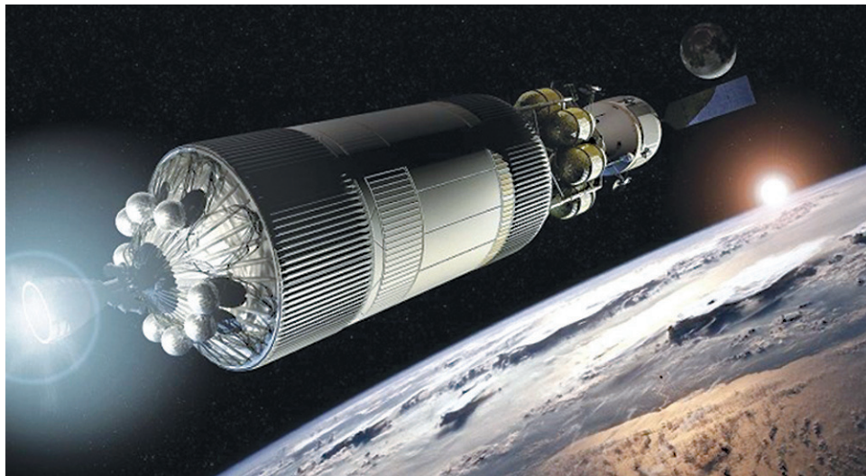
Artist's depiction of an Earth Departure Stage of a proposed NASA Mars mission, docked to the Crew Exploration Vehicle.
