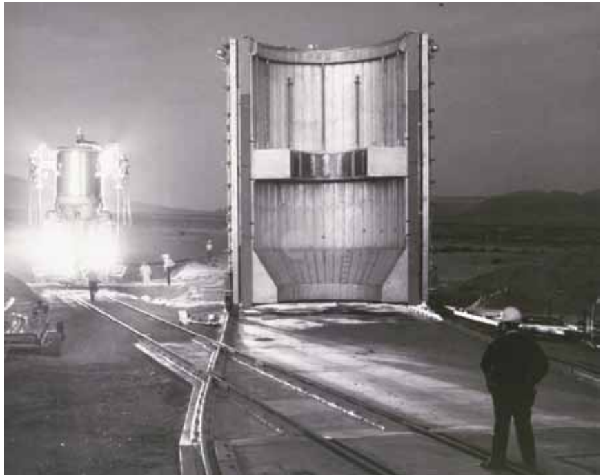
The NERVA-XE, the first ground experimental nuclear thermal rocket engine undergoing testing in 1967.
