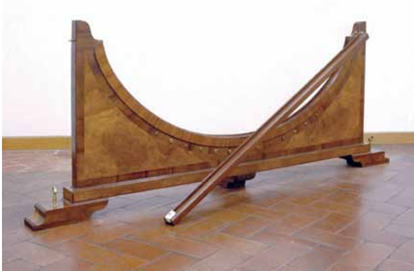
Least action pathways are not always straight lines. A brachistochrone and a pencil in water, illustrate the least action curve of a ball rolling down a track, and the least action refractive angle for light going from air to water.
