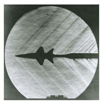
The followers of Descartes and Newton insisted, up until the 1940s, that Riemann was wrong, that transsonic and supersonic flight were impossible. Shown here are shock waves generated by an X-15 model being tested in the NASA/Langley Research Center's Supersonic Pressure Tunnel in 1962.
