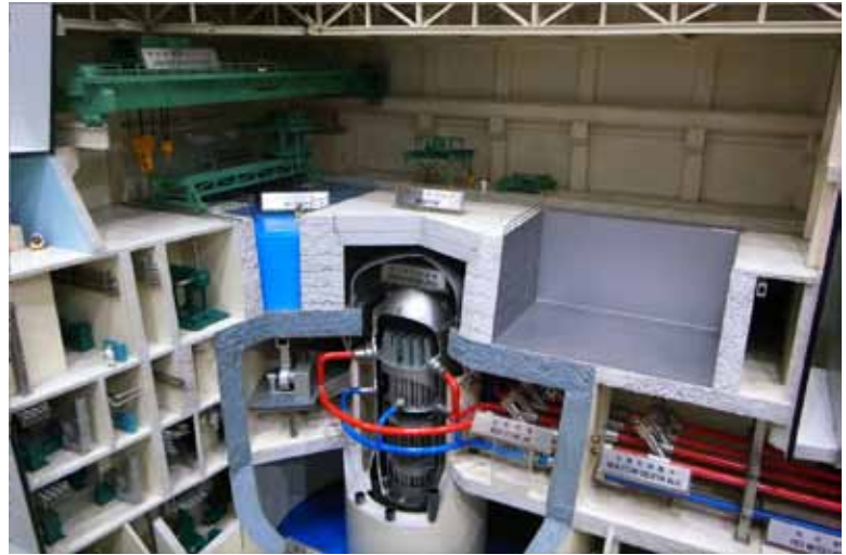
Model of the Toshiba ABWR, which became the first operational Generation III reactor in 1996.
