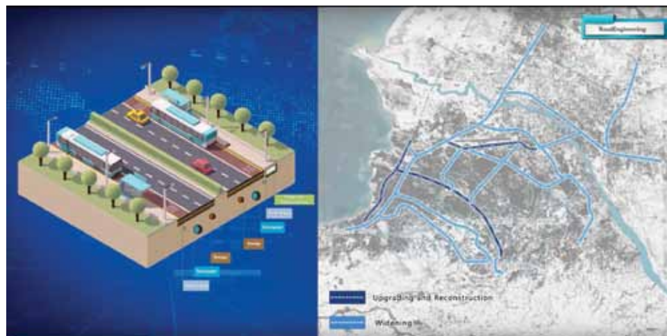
Road drainage with water supply, stormwater, sewage, and power and communication conduits.
