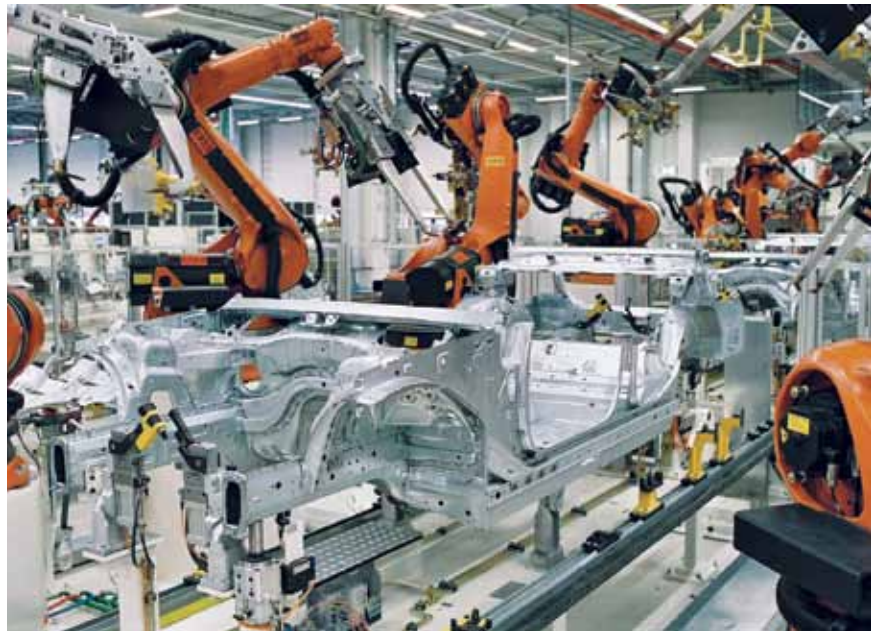
Computer-controlled spot welding in the BMW plant in Leipzig, Germany, 2005, using industrial robots manufactured by KUKA, an Augsburg firm.
