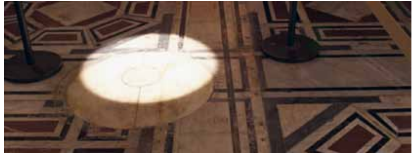
The Renaissance astronomical instrument called the gnomon in the Cathedral of Santa Maria del Fiore, invented in 1475 by Paolo Toscanelli, and restored by Father Leonardo Ximenes in 1754.
