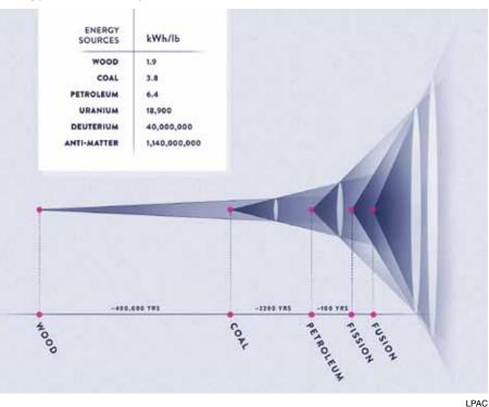
This progression of cones of increasing pitch show the natural progession of sources of fuels of higher energy density. Apexes represent the time of their discovery. As a new cone reaches the previous one, the old technology becomes eclipsed in its use in the economy. Both the rate of discovery, and the relative energy ratios are increasing dramatically. Deuterium is used here as the fuel for fusion reactions.
