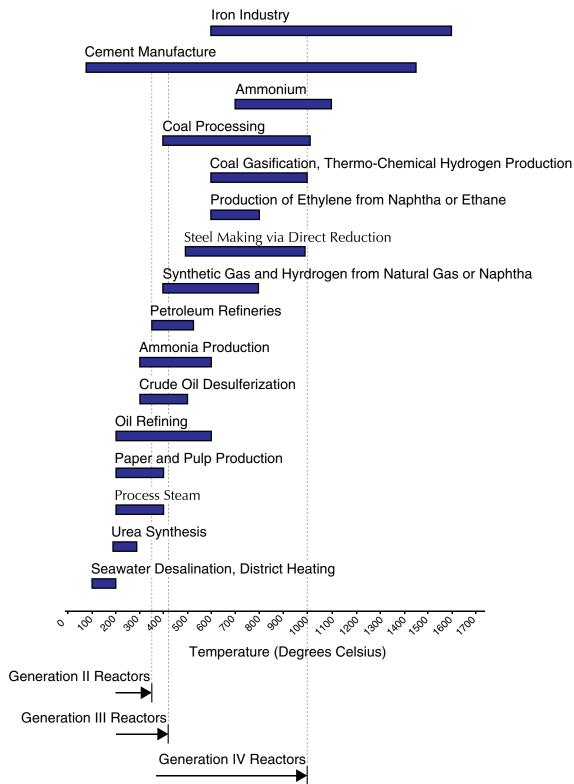
Comparison of common industrial-process heat-temperature requirements, with nuclear-reactor temperatures.<sup>1</sup>
