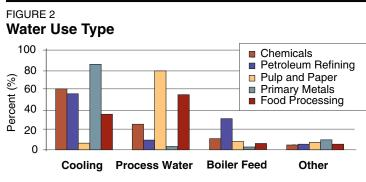
Source: Ellis, Industrial Water Use and Its Energy Implications Breakdown of how each type of industry uses water. Boiler feedwater is water used to supply a boiler to generate steam or hot water.
