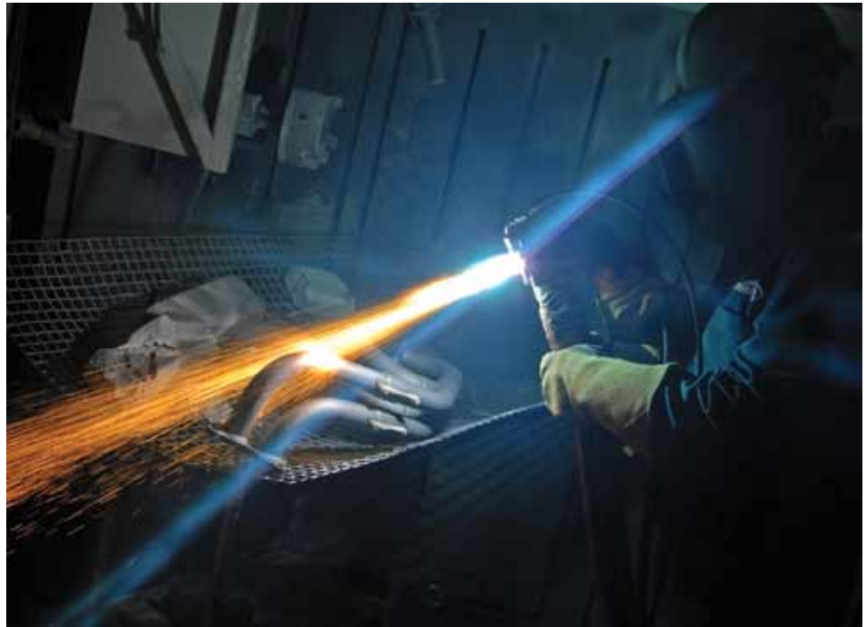
Plasma Thermal Spraying: a plasma torch shoots a jet of plasma (on the order of 10,000°C) into which materials are introduced, melted, and sprayed onto a substrate.
