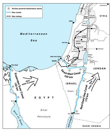
But the idea then is, from the Red Sea, to build a canal, which goes downwards to the Dead Sea, and you can use the difference in elevation for hydropower. The idea was to desalinate water with that power, which Jordan needs a lot. That project is dead. It doesn't exist anymore because of all these political destabilizations. But the engineers are ready to build it.
