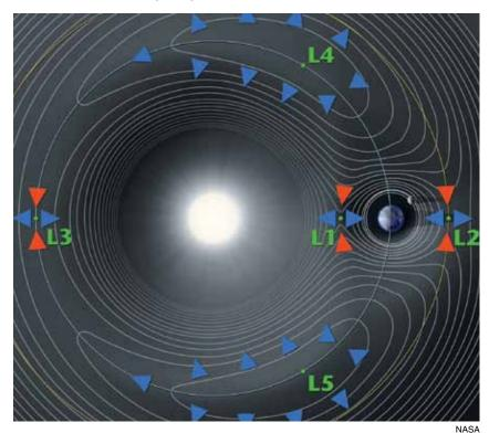
The five Earth-Sun Lagrange points (bodies not to scale) are locations where the gravitational effects of the Earth and Sun reach a type of equilibrium. L4 and L5 are known as stable points, within which small bodies, such as small asteroids or man-made satellites, can maintain an orbit.
