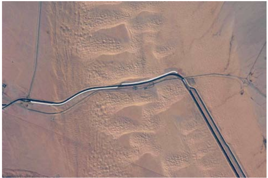
The All-American Canal in Southern California is the largest irrigation canal in the world. It brings water westward from the Colorado River to irrigate the Imperial Valley and supply water to nine cities. The dark line is the canal, which is crossed in this image by Interstate 8.
