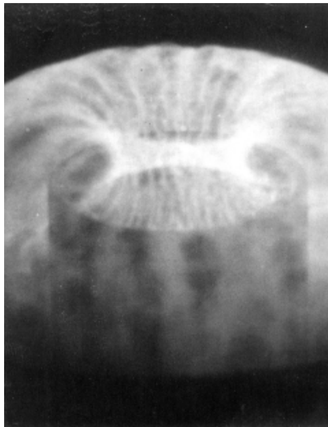
Vortex filaments from the current sheath in a plasma discharge from a theta pinch fusion machine, photographed by Winston Bostick. The filaments show the natural tendency of a plasma toward organized structure.
