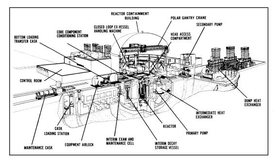
The FFTF is a liquidsodium-cooled reactor with a fuel of mixed uranium oxide and plutonium oxide. Fast flux refers to the speed of neutrons produced in the reactor core during the fission process. The reactor vessel is located in the domeshaped containment building.
