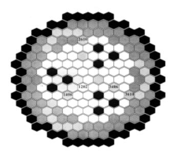
This schematic of the FFTF core with multiple missions shows the hexagonally shaped ducts, in which multiple experiments can be conducted. Some ducts contain the fuel rods and control rods. Others are for isotope production, fuel tests, and so on.
