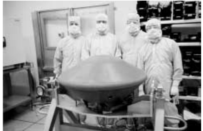
The diminutive size of the 130-pound landing capsule, with Beagle 2 tucked inside it, is evident, as seen here, before shipment to be integrated with Mars Express.
