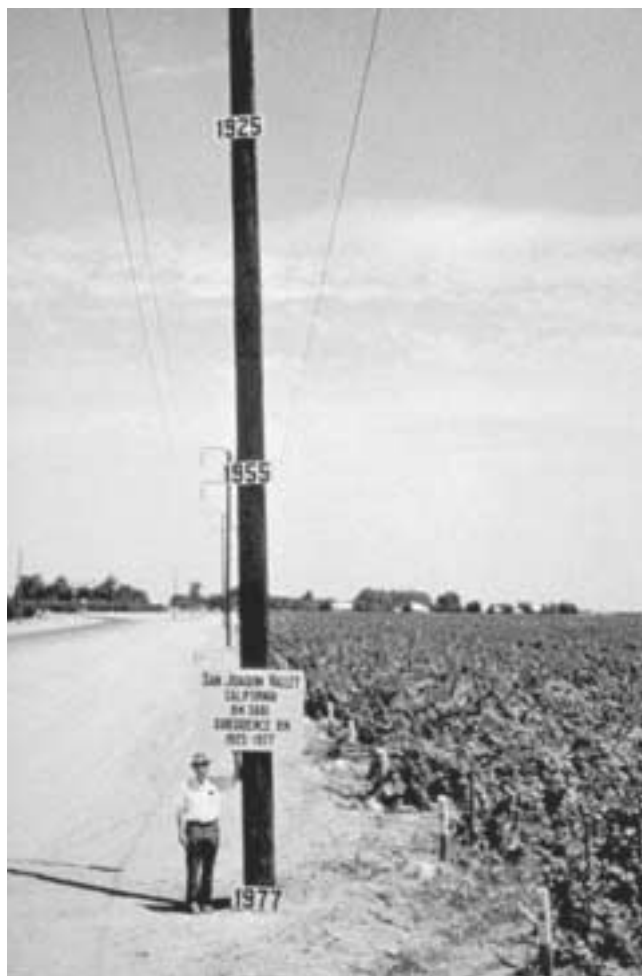
Prof. Endersbee in California's San Joaquin Valley, next to a pole recording the approximate level of the farmland at three times in the 20th Century; the land had subsided about 30 feet, due to the groundwater underneath it being exhausted and not replenished.
