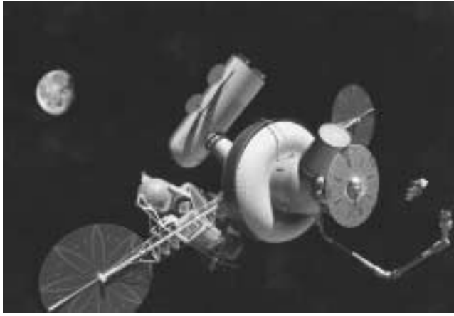
NASA's Exploration Team has proposed that a "Gateway" facility be built at the Earth-Moon L1 point, 322,127 kilometers (about 190,000 miles) from Earth. The Gateway would include temporary living quarters for visiting crew, facilities to service astronomical observatories, and vehicle fueling and servicing centers for journeys to the Moon and Mars.
