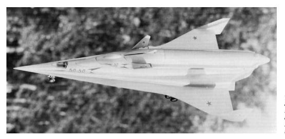
The Soviet "Spiral" aerospace plane, which included a hypersonic airplane booster and small orbital plane on top.
