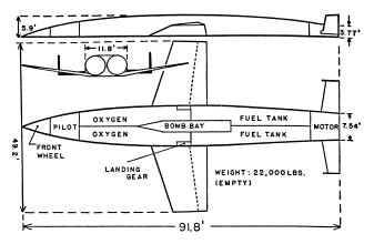
A diagram of Eugen Sänger's anti-podal bomber, which would be capable of travelling halfway around the world and landing at an airport.
