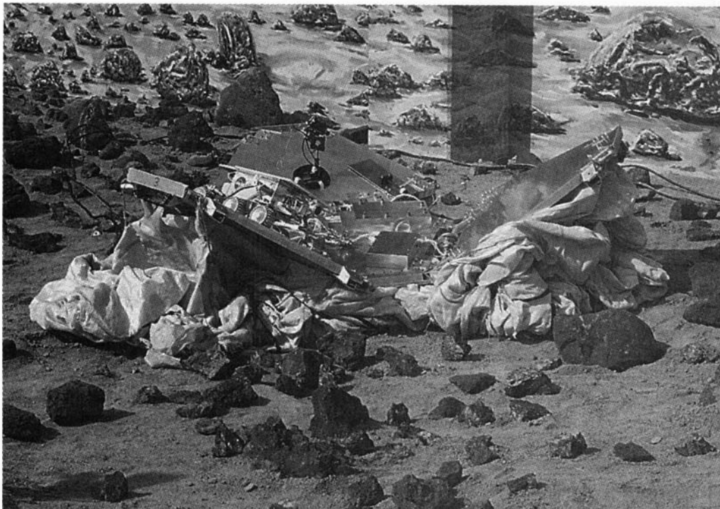
After the Mars Pathfinder lander is on the planet's surface, its air bags will deflate, and the three petals protecting the scientific instruments will open. Nestled on one of the petals will be the tiny Sojourner microrover (left petal), which will collect data and relay it back to the lander, for transmission to Earth.
