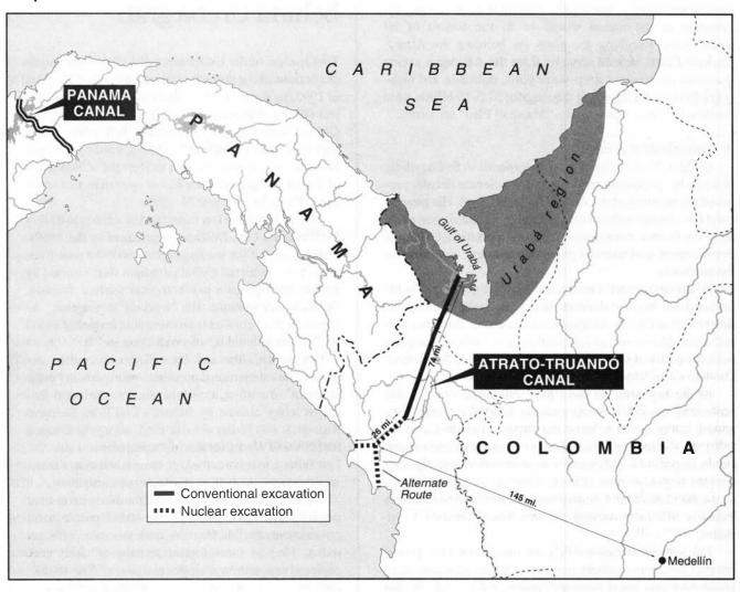
250,000-ton tankers were navigating the globe. The U.S. Army Corps of Engineers recommended the peaceful use of nuclear energy as a means of building a new canal. It was estimated that 19 nuclear explosions would be required, along 26 kilometers of rocky mountains; along the remaining 185 kilometers, conventional excavation technology could be used. The canal would have a good two-way course, at sealevel (without locks), and would operate year-round.
