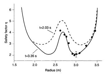
Safety factor q profiles for TFTR at two different times, center of core is at approximately 2.65 radii on the major radius. The two low points of the W-shaped curve are where the shear reverses.
