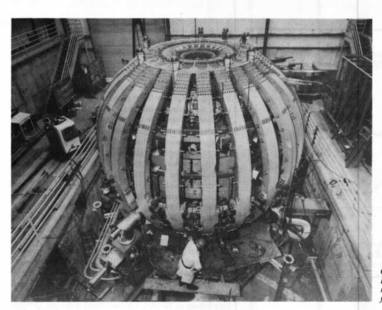
General Atomics' Doublet III-D tokamak magnetic confinement fusion device.
