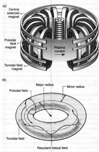
This artist's rendition of a typical tokamak fusion device (a), shows the magnets and plasma current. The bottom schematic (b) shows the configuration of the magnetic fields within a tokamak, in which the magnetic fields confine and heat plasma inside of a donut-shaped vacuum chamber. Within the plasma, the toroidal and poloidal magnetic fields combine to produce helical fields.
